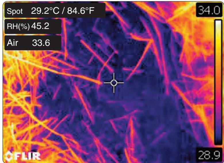
Concrete temp from adequate pre-heating and the minimum ventilation system transporting the warm air uniformly.
