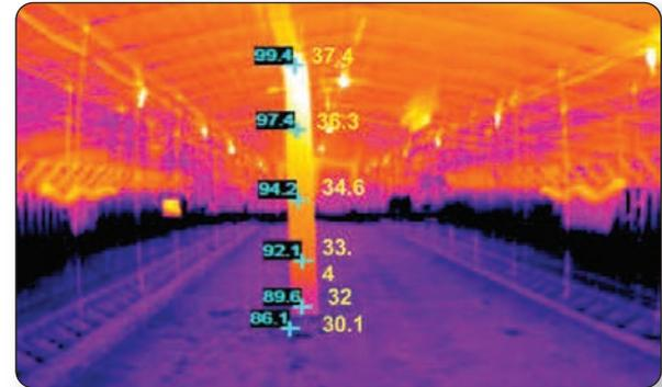
Reduction in RH% when air is heated to 30°C (86°F)
