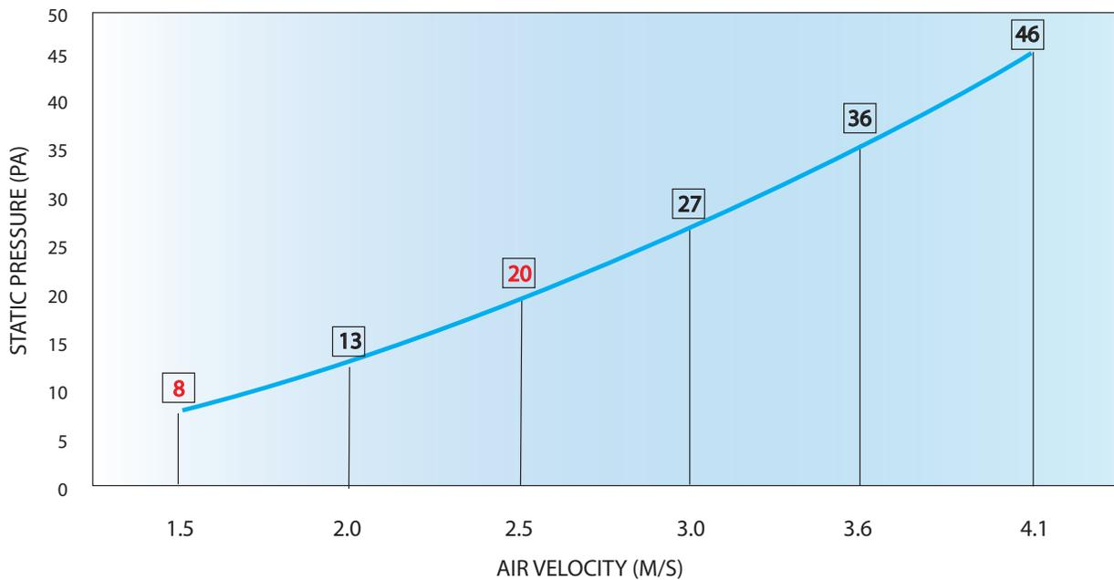
The tunnel inlet light trap was sized at 1.5 m/s (300 fpm) with a pressure drop of 8 Pa (0.03 in wc). The tunnel fan light trap was sized at 2.5 m/s (500 fpm) with a pressure drop of 20 Pa (0.08 in wc). (See the values highlighted in red)
