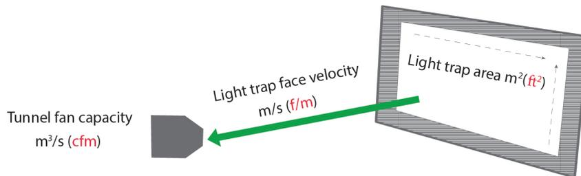
$$\text{Light trap area m}^2 \text{ (ft}^2\text{)} = \text{Tunnel fan capacity m}^3/\text{s (cfm)} \div \text{Light trap face velocity m/s (f/m)}$$
