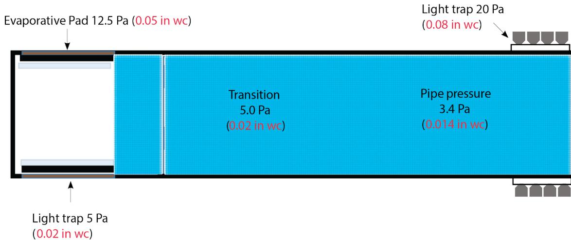
**Total fan operating pressure *with* evaporative pads 45.9 Pa (0.18 in wc)**
