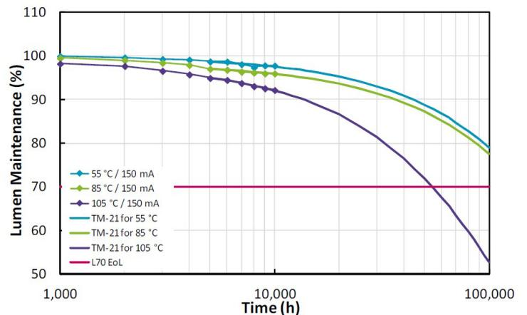
Note how the 105°C LED drops below the 70% before the 55/85°C LED in this example.
