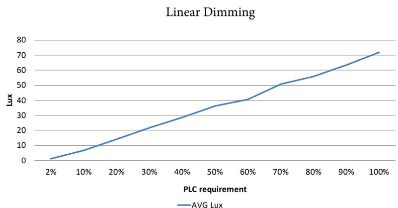
*A linear dimming curve makes for simple programming of your PLC: 0V = Off, 5V = 50% and 10V = 100% output.*
