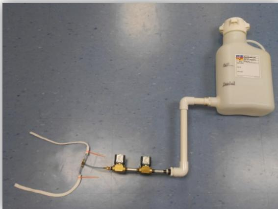
**Figure 3:** An automated system where a clock and pumps are used to automatically release formaldehyde at prescribed intervals without human interaction.
