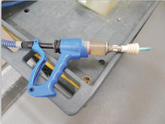
**Figure 1:** A hand held device where the dosage can be changed with a dial. The end of this device is placed at an insertion point on the hatcher cabinet to then place formaldehyde into the cabinet.
